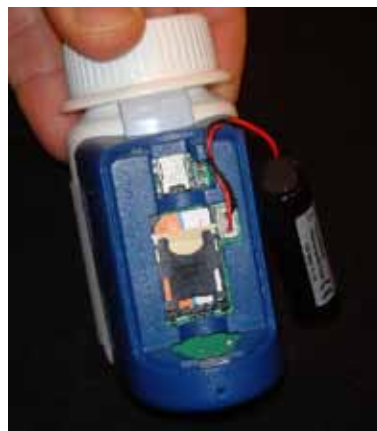
A SIMpill bottle's SIM card and transmitter
