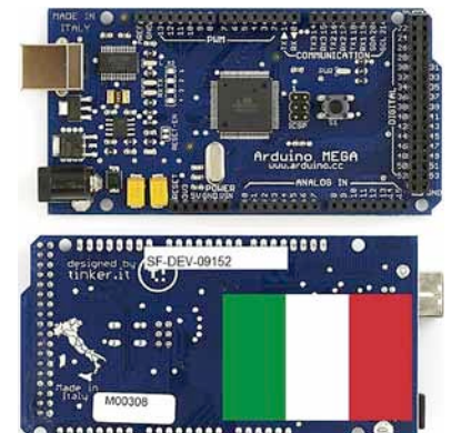
Arduino, an open-source electronics prototyping platform based on flexible, easy-to-use hardware and software, was designed in Italy but likely assembled elsewhere.
