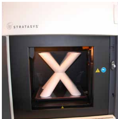
Fused deposition modeling prints by depositing layers of material.
