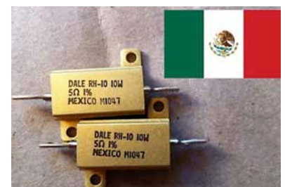
The power resistors, from Mexico, are responsible for heating the nozzle that distributes the melted plastic.
