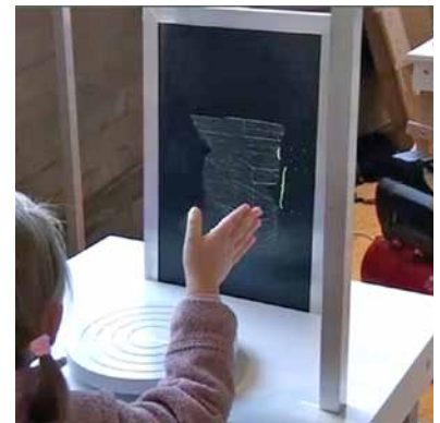
The RepRap virtual pottery wheel allows users to directly shape objects for printing.
