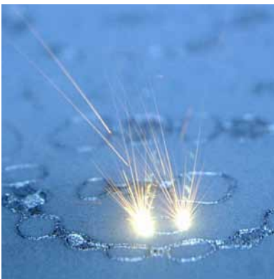
Laser sintering melts layers of fine metal filings into a solid object.
