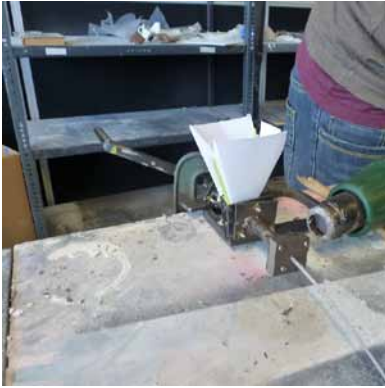
The Recyclebot allows users to use shredded milk bottles as feedstock.
