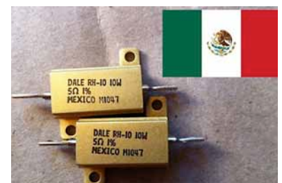
The power resistors, from Mexico, are responsible for heating the nozzle that distributes the melted plastic.
